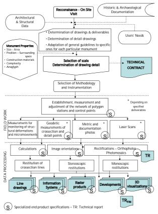
Figure 7 Steps for carrying out the geometric documentation of a monument
